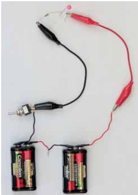
Figure 3: A circuit with an LED, a battery, a switch and a resistor
