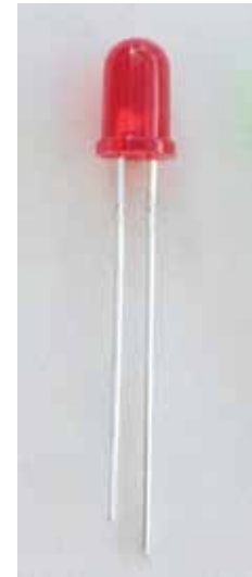
Figure 12: An LED. The longer of the two wires coming out of the LED should be connected to the positive terminal, and the shorter wire to the negative terminal.
