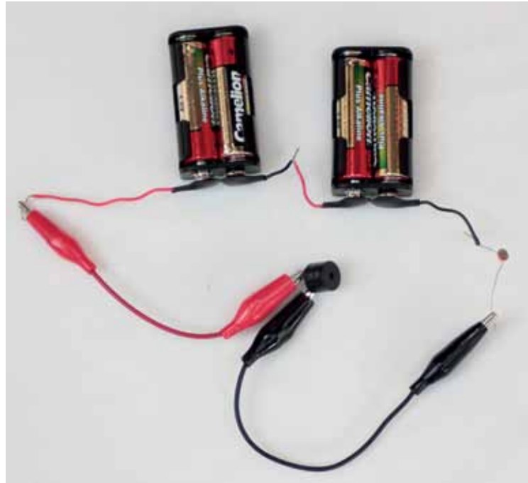
Figure 4: A circuit where the current is regulated by a light-dependent resistor
