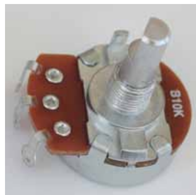
Figure 3: The control knob of a stove plate is connected to a variable resistor. This controls the current through the heating element. The bigger the current, the hotter the plate will be.
