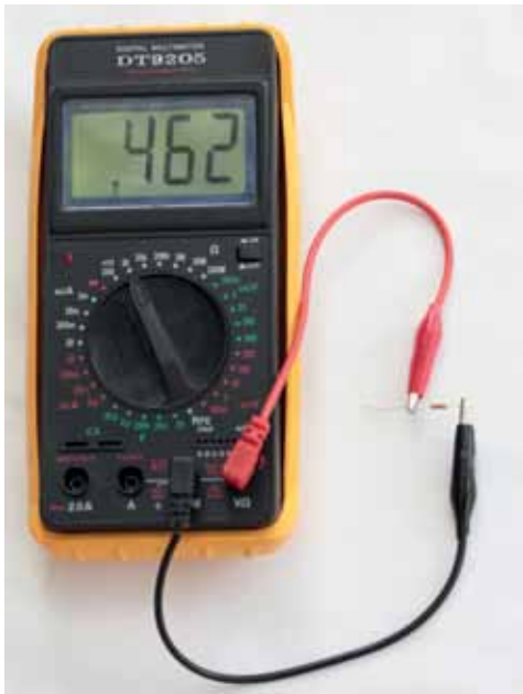
Figure 17: Multi-meter set and connected to measure resistance
