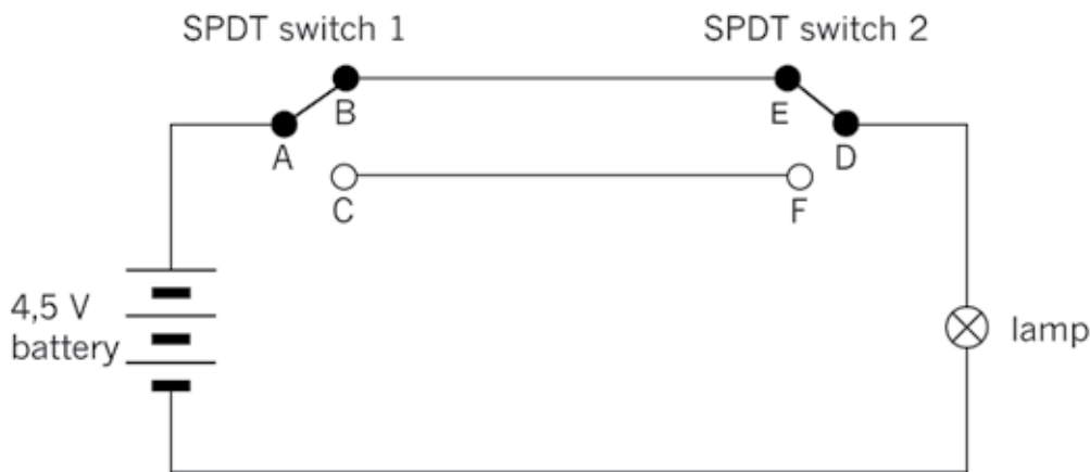
Figure 7: A circuit with two SPDT switches is often used to control a lamp with one switch at each end of a long passage. It is also used to control a lamp with one switch at the bottom of a staircase, and the other switch at the top of the staircase.
