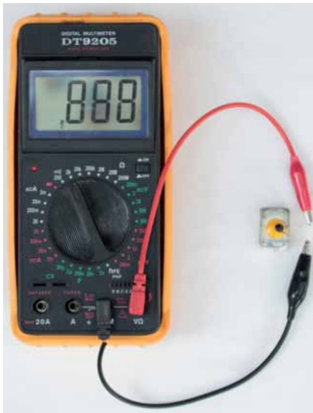
Figure 3: Measuring the resistance of a thermistor while heating it with a hot object. You can heat a metal thumb tack by pressing it into an eraser, and then rubbing it hard against a piece of wood or plastic for one minute.
