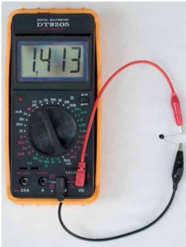
Figure 2: Measuring the resistance of a thermistor at room temperature.
