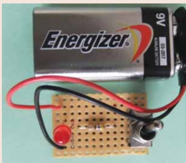
Figure 10: A simple LED circuit built on a strip board
