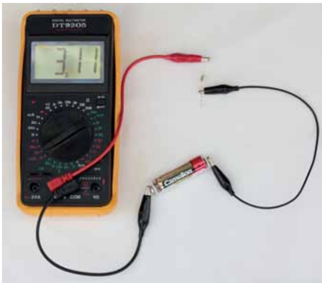
Figure 18: Multi-meter set and connected to measure current
