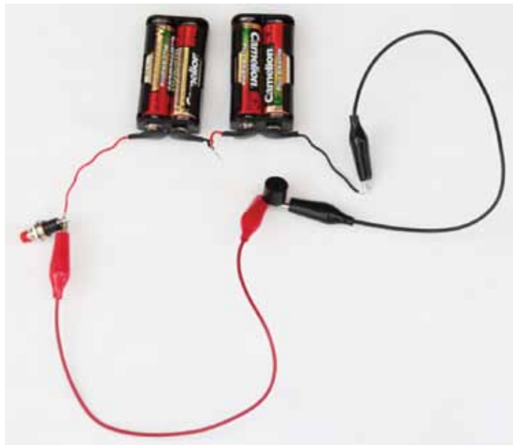
Figure 2: A simple doorbell circuit
